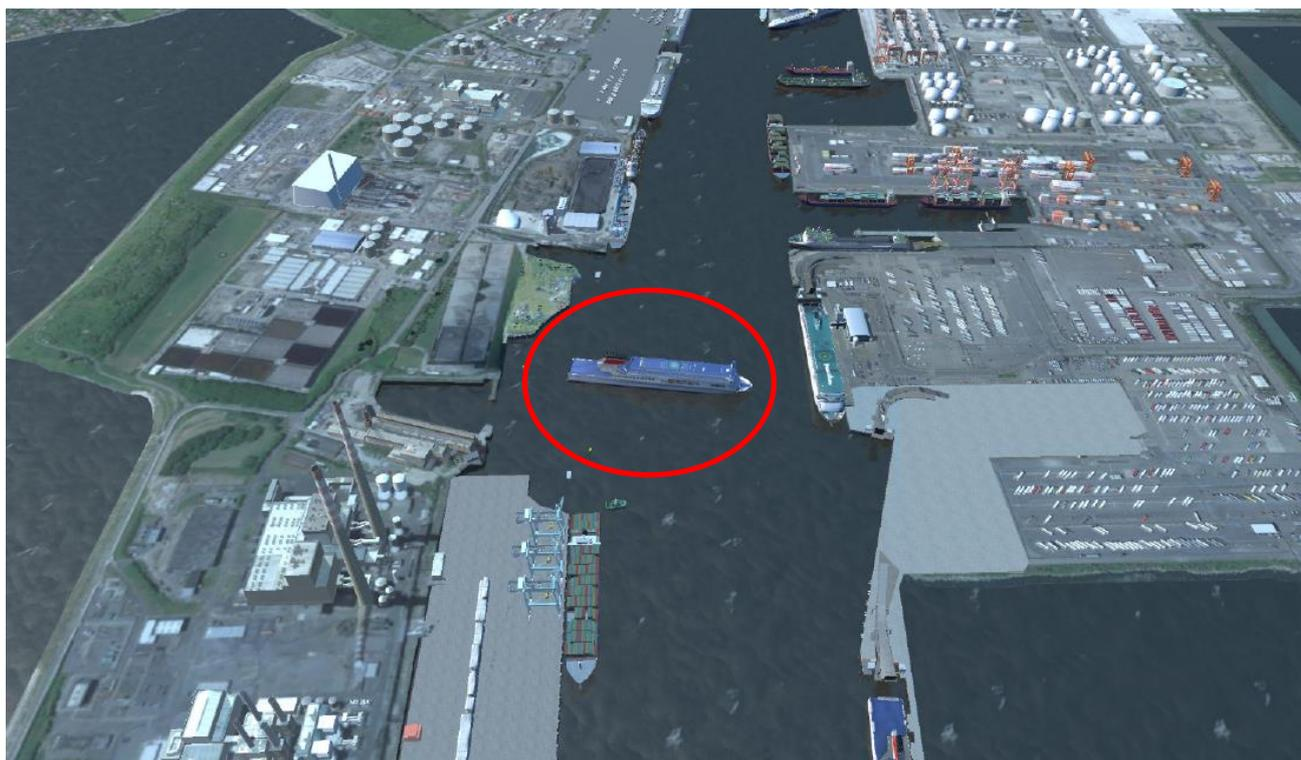
Figure 5.21 Example visual scene from HR Wallingford's Ship Simulator, illustrating the Turning Circle in use. Turning Circle shown indicatively in red. View looking west.
