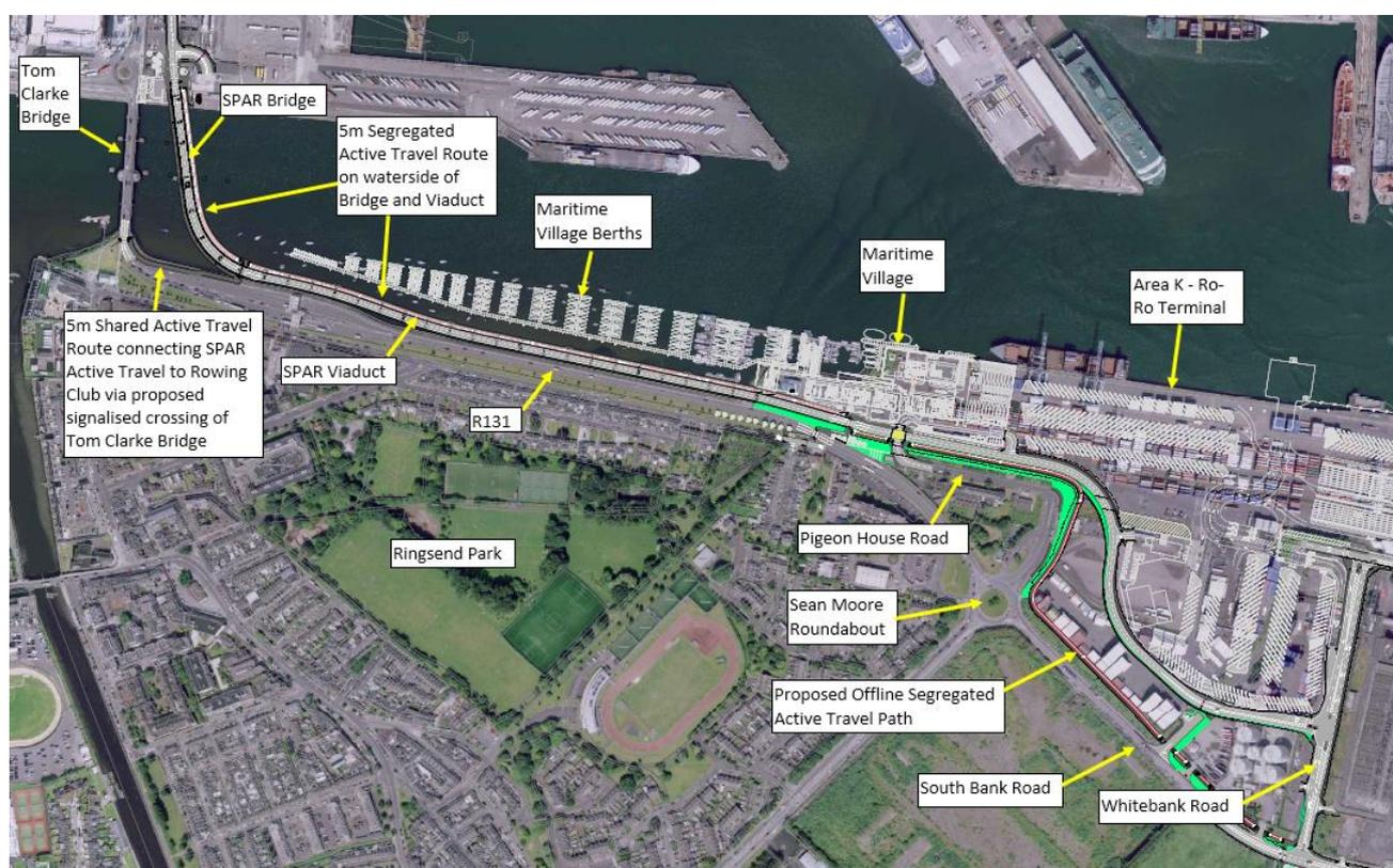
Figure 5.10 SPAR Bridge and Viaduct and connection to Whitebank Road
